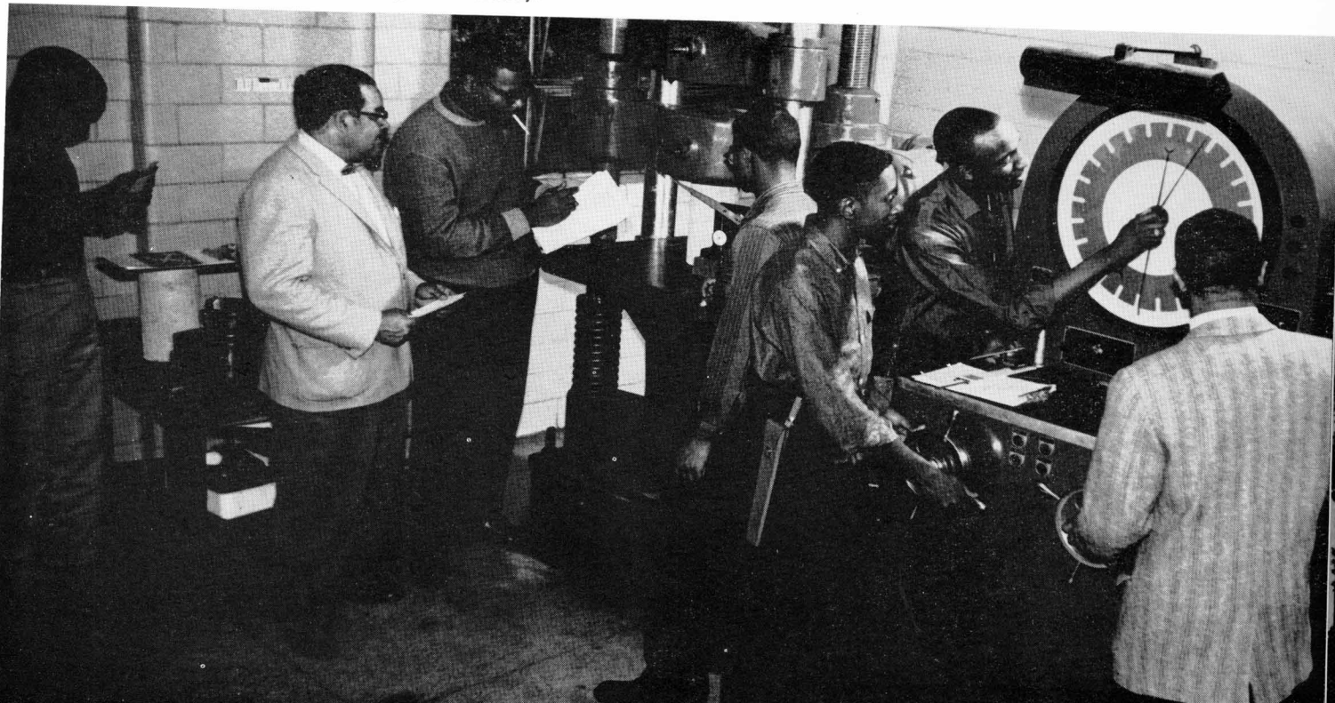
Laboratory tests to determine sheaving resistance and unconfined compression are made in the civil engineering soils laboratory.
